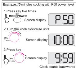
Note:1. The power level is displayed in the percent. With each pressing of the key MICROPOWER the power level reduces from p100 to P80 to P70to P60to P50 to P40to P30 to P20 then start again from P100.
